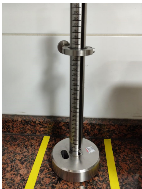
Fig. 3. The small ball test ( AC3 \geq 10 mm, BS-EN 13329+A1 [4])
