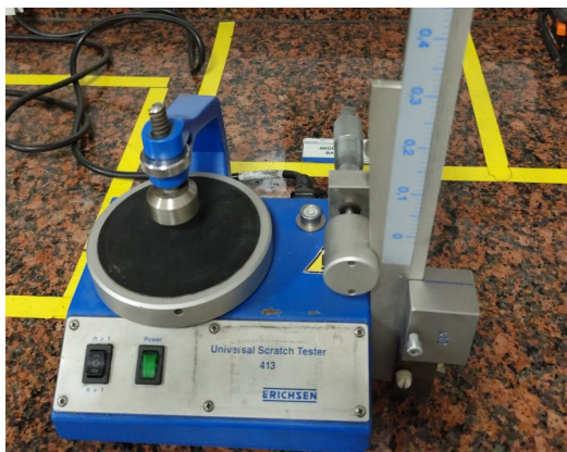
Fig. 2. The scratch resistance test
