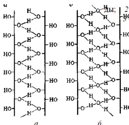
Fig. 4. Diagram of bridge bonds between parallel pulp chains: *a* – chains joined by lateral bonds using hydrogen bridges in dry fibre, *b* – chains joined by water molecules using water bridges in wet fibre
