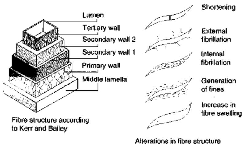
Fig. 7. Possible impacts on fibres during pulp treatment
