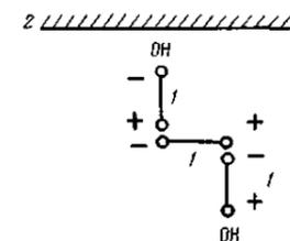
Fig. 3 Diagram of interfibre bridge bonds based on water dipoles: 1 – water dipoles, 2 – first fibre, 3 – second fibre.
