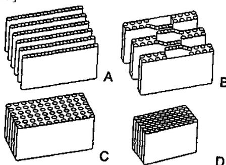
Fig. 1. Changes in the fibre wall structure [25]: A–D – drying stages
