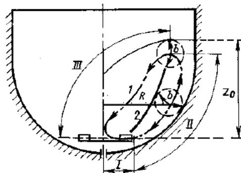
It was accepted that the flow in the pulper vat formed a closed circuit built on the basis of the above idea of the process physics.
